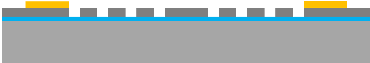
Mask # 2 – Device layer (SOI) etch
