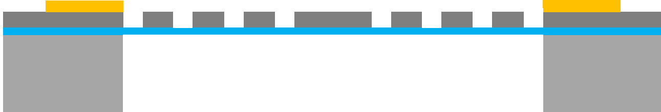
Mask # 3 – Backside trench etch
