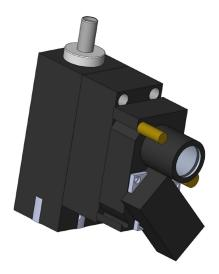
The optical unit is primarily designed for Laser induced fluorescence measurements in Capillary electrophoresis but can also be used in the investigation of materials. The system is a stand alone unit with a laser excitation source and photo multiplier detection system on board. The operators system must provide a 0 to 1 volt input to set the photo multiplier gain and must input the signal into their data acquisition system. [0 to 5 vdc]
