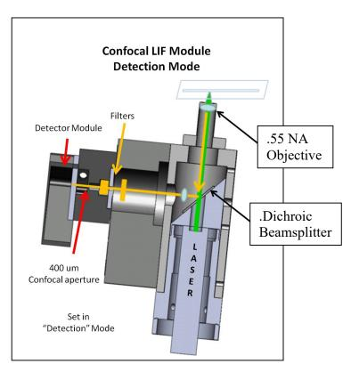
controls the PMT gain. The microscope unit is equipped with a mechanical switch, "turret" which allows the user to view through the microscope, focus the image and center the laser spot onto the point of interest in the Capillary. The switch is placed into the detection position, and the unit is ready to collect data.
