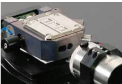
Laser head (inside view) with pro technology ECDL resonator.
