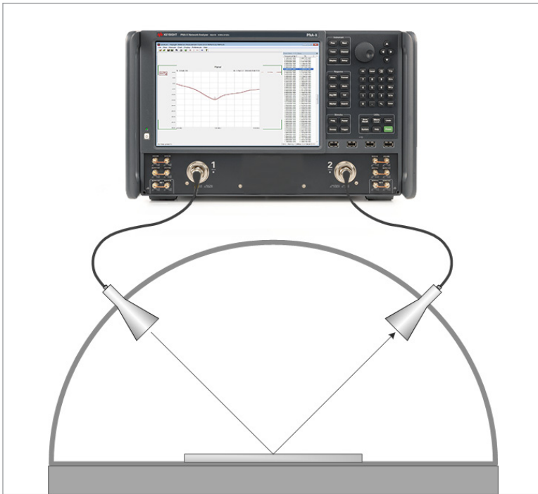
Figure 7. In the NRL arch method, one antenna transmits energy onto the MUT and the second antenna receives the reflected portion.
