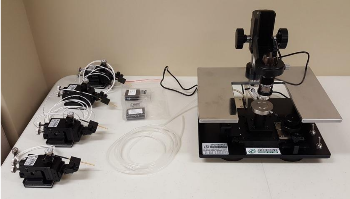
Figure 2: Probe Station and Positioners Ready to Be Configured (Microscope Installed, Vacuum Pump and Hex Keys Not Shown)
