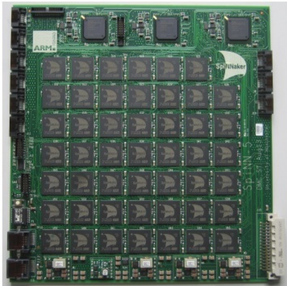
The SpiNNaker Board: A building block of a SpiNNaker machine, containing 48 chips for a total of 864 ARM processors.
