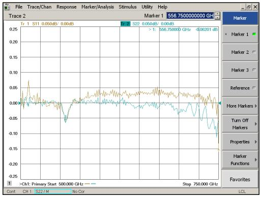
Figure 3. Typical drift performance of the PNA/PNA-X solution at 500 to 750 GHz with Virginia Diodes frequency extenders
