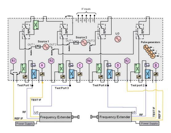
Configuration of a banded solution is similar to configuration of a single sweep solution using separate components. With the support of several frequency extenders and vector network analyzer options, the banded solutions, offer industry leading flexibility and extensibility for measurements to 1.5 THz.
