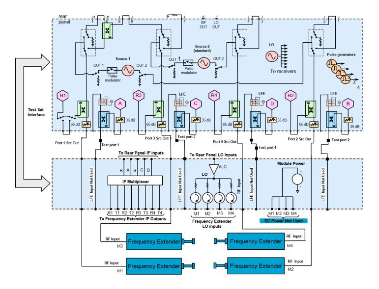
These solutions do not require a millimeter-wave test set controller as they connect directly to the front panel of a dual source PNA or PNA-X. Both VDI and OML frequency extenders are supported with this configuration. Here is an example of a set of VDI modules that are directly connected to a dual source PNA.
