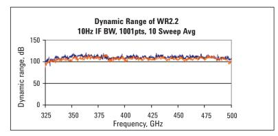
Figure 1. Dynamic range of a 325 to 500 GHz WR 2.20 VDI frequency extender
