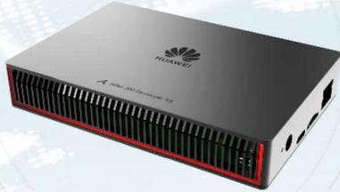
The Atlas 200 DK (model: 3000) is a high-performance AI application developer board that integrates the Ascend 310 AI processor to facilitate quick development and verification. It has been widely used in scenarios such as developer solution verification, higher education, and scientific research.
