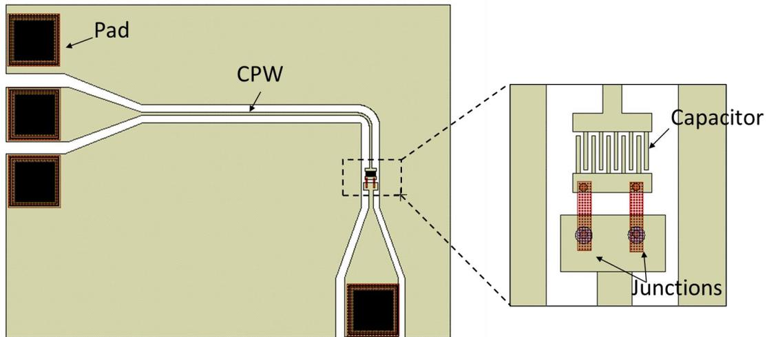
Figure 5: A quantum circuit designed using the CMC Cell Library and Siemens EDA's L-Edit.
