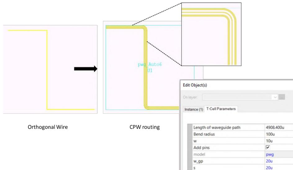
Figure 4: An orthogonal wire drawn is converted to a CPW routing. The parameters of the routing can be modified in the “Edit Object” window.
