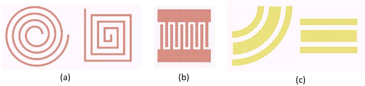
Figure 3: Examples of P-cells: a) Spiral and square inductors b) Finger capacitor c) CPW bend and straight waveguide.
