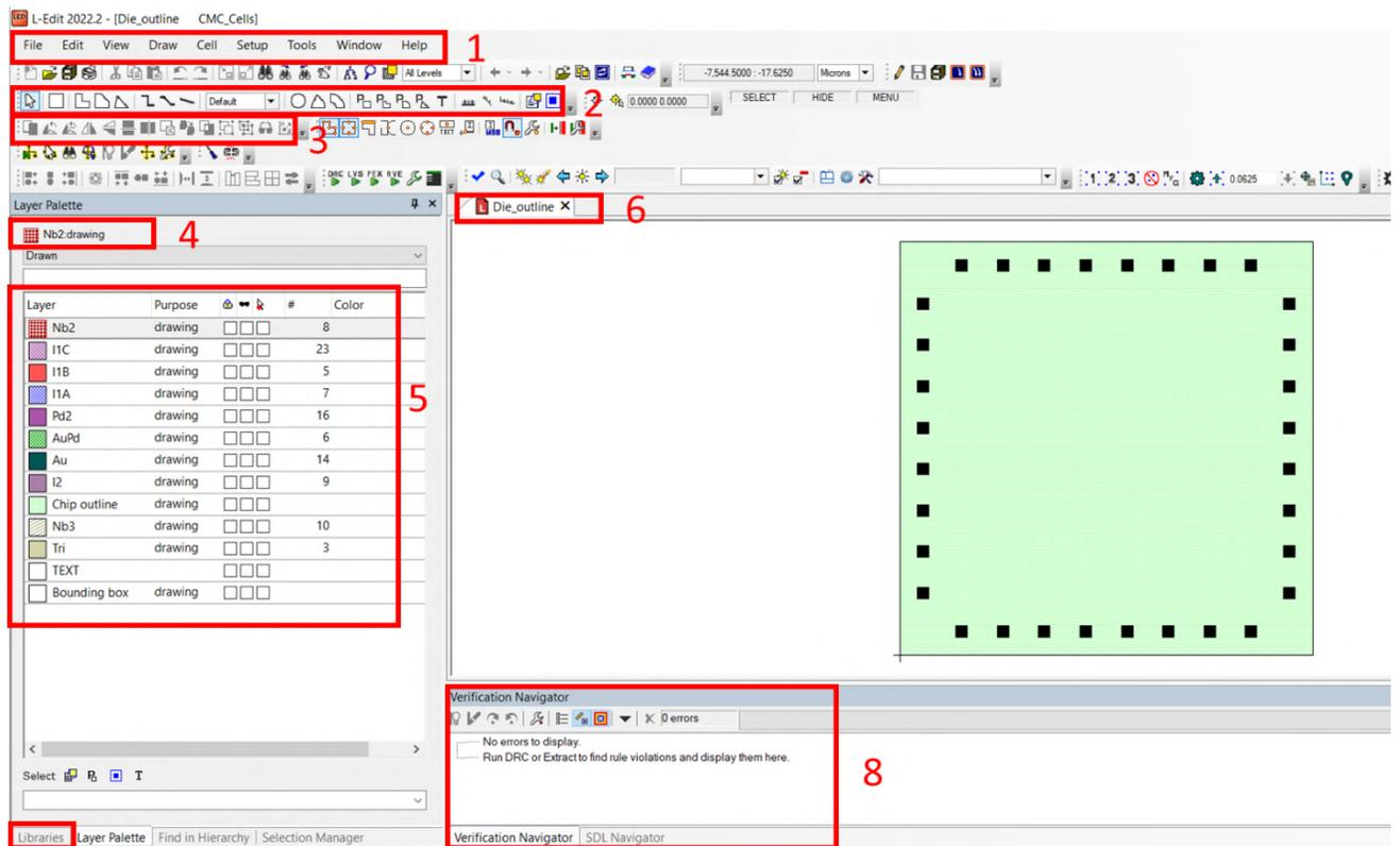
Figure 1: L-Edit main window and useful features such as Main (1), Editing (2) and Drawing toolbars (3), Current layer (4), Layer Palette (5), Current cell (6), Libraries (7) and Verification navigator (8).
