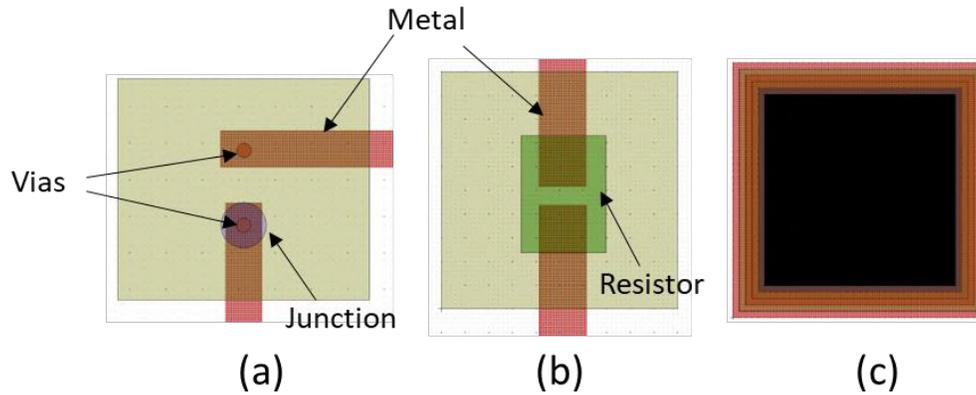
Figure 2: Examples of reference layout cells: a) circular Josephson junction, b) resistor, and c) pad.
