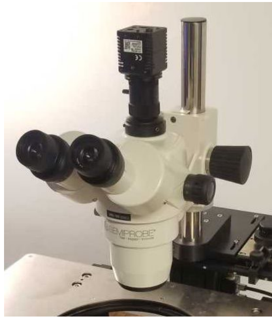
Figure 12 – Remove dust cap and install camera with label forward for upright image. Camera ring has hex screws and thumbscrew to securely mount camera. Do not overtighten.
