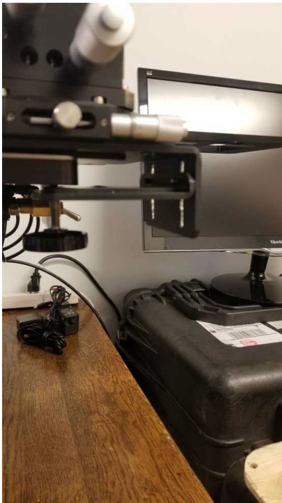
Figure 30 – Left: The clamp bracket tightening screw is right at the edge of the platen. Right: With both positioners installed, the probe station setup is almost complete.
