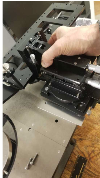
Figure 26 – Remove the hex screws, align the shim and mount the positioner. Use the hex screws to secure the positioner to the platen.
