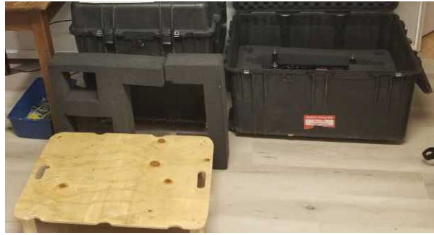
Figure 19 – Once the top layer boxes and vacuum pump are removed, remove the foam and shelf.
