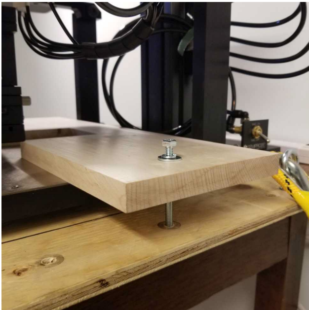
Figure 6 – The bolts for these retaining boards are a specific length not to protrude too far through the lower board as it sits directly on the bottom of the case. Remove for setup, and when reinstalling, the boards may need to be squeezed together to start the threads.
