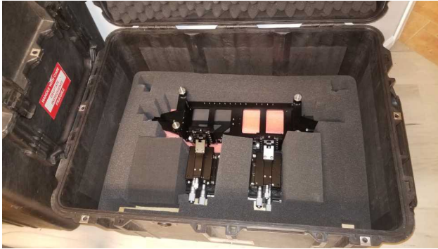
Figure 20 – Remove the foam protecting the positioners. The positioners are securely attached to the platform. When lifting out the platform of positioners, note that the brackets extend below the platform, so it will need to be placed on blocks. See next figure.
