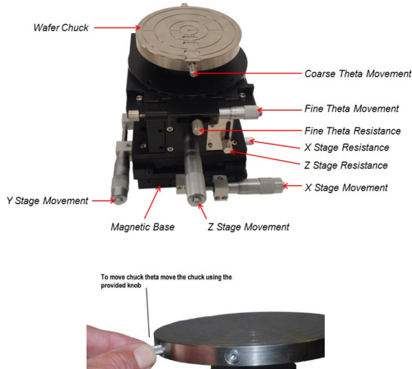
Figure 37 – Left: From pg 13 & 17 of “LA-50 - LA 200 Operating Manual.pdf” Right: thumbscrew in circle connects or releases the rotational stage to the micrometer. The thumbscrew in the square locks the rotational stage once it is in the right position.
