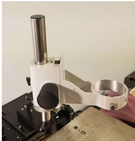
Figure 9 – Install and tighten the microscope tube on the station, then add the focus block.
