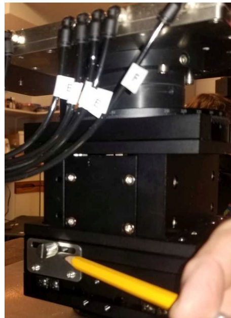
Figure 35 – Left: thumbscrew circled beside the rotational micrometer connects the micrometer to the stage. The magnetic base is enabled when lever is moved to the right. Move to the left to reposition the stage on the base plate.
