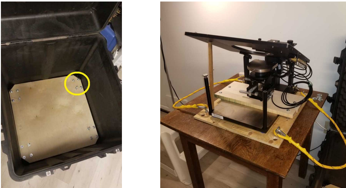
Figure 3 – Left: Board at bottom of case has long protruding bolt in each corner.
