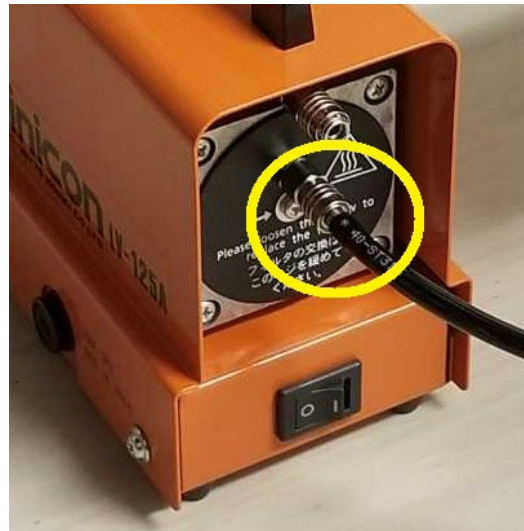
Figure 32 – The station vacuum tubing is coiled and attached to the side of the microscope stand. Uncoil it and plug the tube into the front center port of the vacuum pump. It is a push-on quick-release connector. To release the tubing for packing up, pull on the cylindrical outer collar of the connector.
