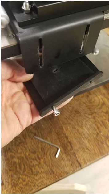
Figure 29 – Attach the positioner clamp bracket to the positioner clamp with the hex screws.
