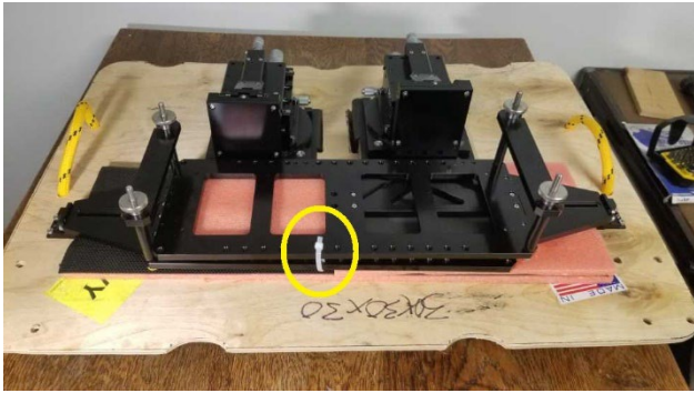
Figure 23 – These positioners are large form factor to hold the VNA frequency extension modules. After being secured to the platform for shipping, the positioner carriages are tie wrapped together.
