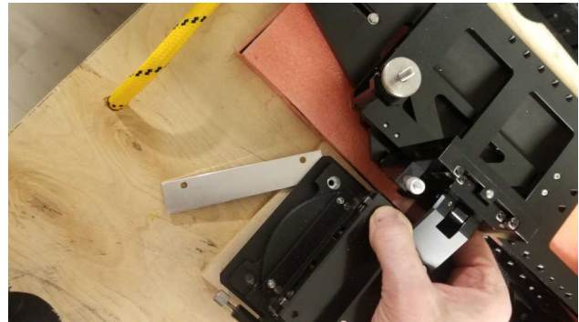
Figure 24 – To begin removal for setup, remove the tie wrap and remove the screws securing the positioner to the case. Note that there is a shim under the positioner base which will be required on the probe station.
