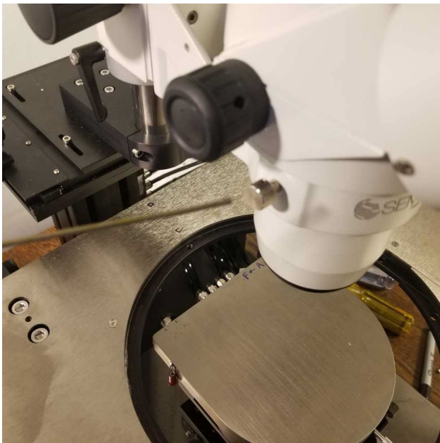
Figure 13 – Left: This pullrod switches between binocular eyepiece and camera views. Right: Route cables so as not to torque camera or the view will be skewed. See notes at end.
