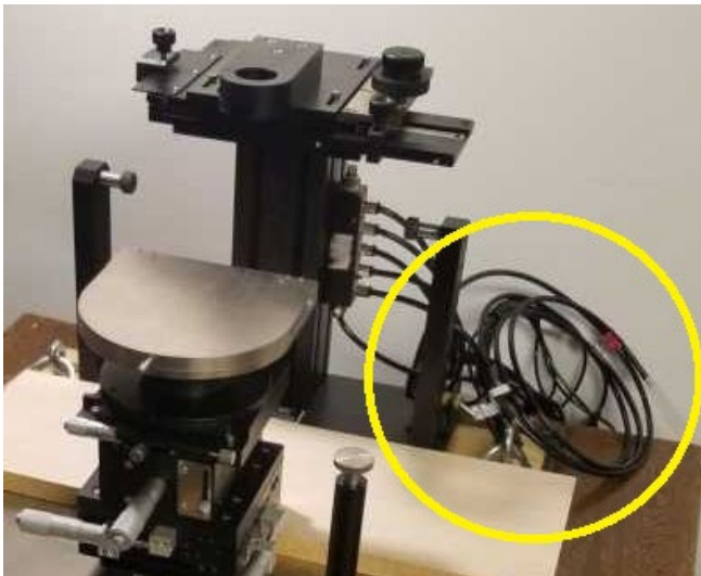
Figure 32 – The station vacuum tubing is coiled and attached to the side of the microscope stand. Uncoil it and plug the tube into the front center port of the vacuum pump. It is a push-on quick-release connector. To release the tubing for packing up, pull on the cylindrical outer collar of the connector.
