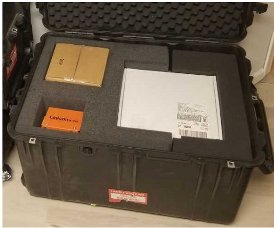
Figure 16 – Top layer of case has a box of accessories, a box of manuals & tools, and the vacuum pump. Brown box contains cables, accessories, positioner brackets, tape and tie wraps.
