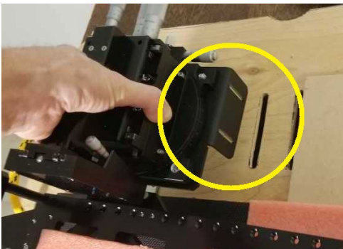
Figure 22 – When removing the positioners in the following steps, you will see that the brackets go through the platform. There are corresponding slots in the bottom foam of the case to accommodate this.
