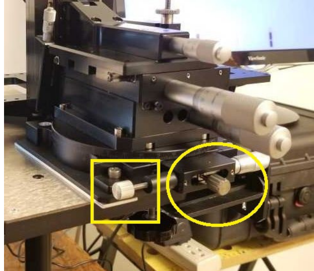
Figure 37 – Left: From pg 13 & 17 of “LA-50 - LA 200 Operating Manual.pdf” Right: thumbscrew in circle connects or releases the rotational stage to the micrometer. The thumbscrew in the square locks the rotational stage once it is in the right position.
