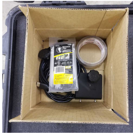
Figure 16 – Top layer of case has a box of accessories, a box of manuals & tools, and the vacuum pump. Brown box contains cables, accessories, positioner brackets, tape and tie wraps.
