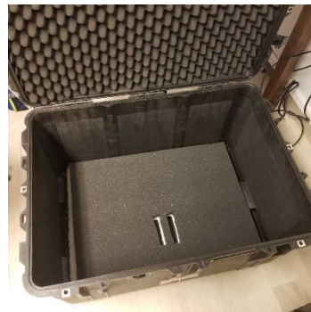
Figure 22 – When removing the positioners in the following steps, you will see that the brackets go through the platform. There are corresponding slots in the bottom foam of the case to accommodate this.
