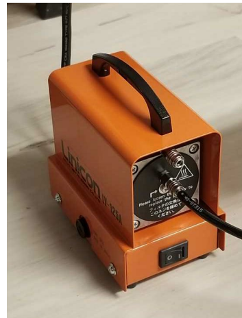
Figure 31 – The final step in the station setup is to install the vacuum pump. Then, the station will be ready to begin the measurement setup – installing probes, adjusting the probes to be planar and calibrating the test instruments.
