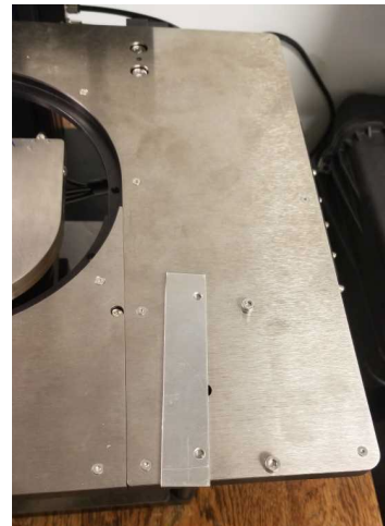
Figure 25 – These shims will be required on the probe station. The mounting hex screws are on the station platen.
