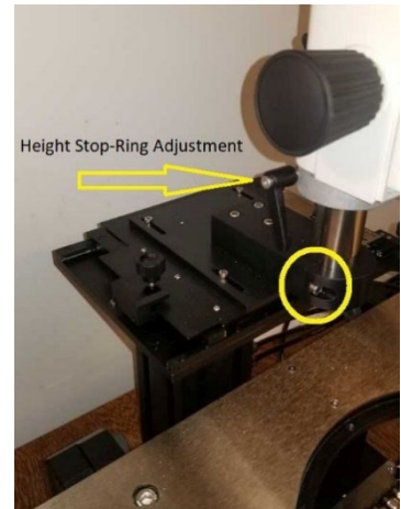
Figure 9 – Install and tighten the microscope tube on the station, then add the focus block.
