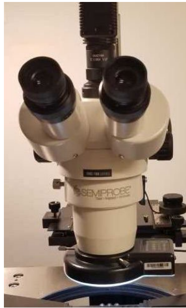
Figure 14 – attach the ring light to the camera lens. Note that the light has a dimmer dial.
