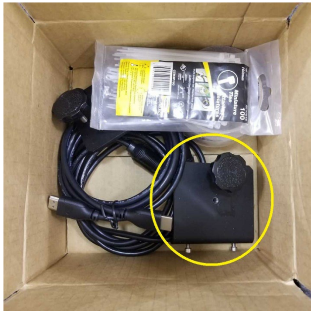
Figure 27 – The shim is required so that the positioner base, which has a rubber bottom, does not tilt forward when tightened. The accessory box has the clamp brackets required to be attached to the positioner bracket.
