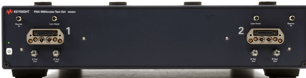
Figure 2-8 N5292A Option 400 (4-Port) Front Panel Features
