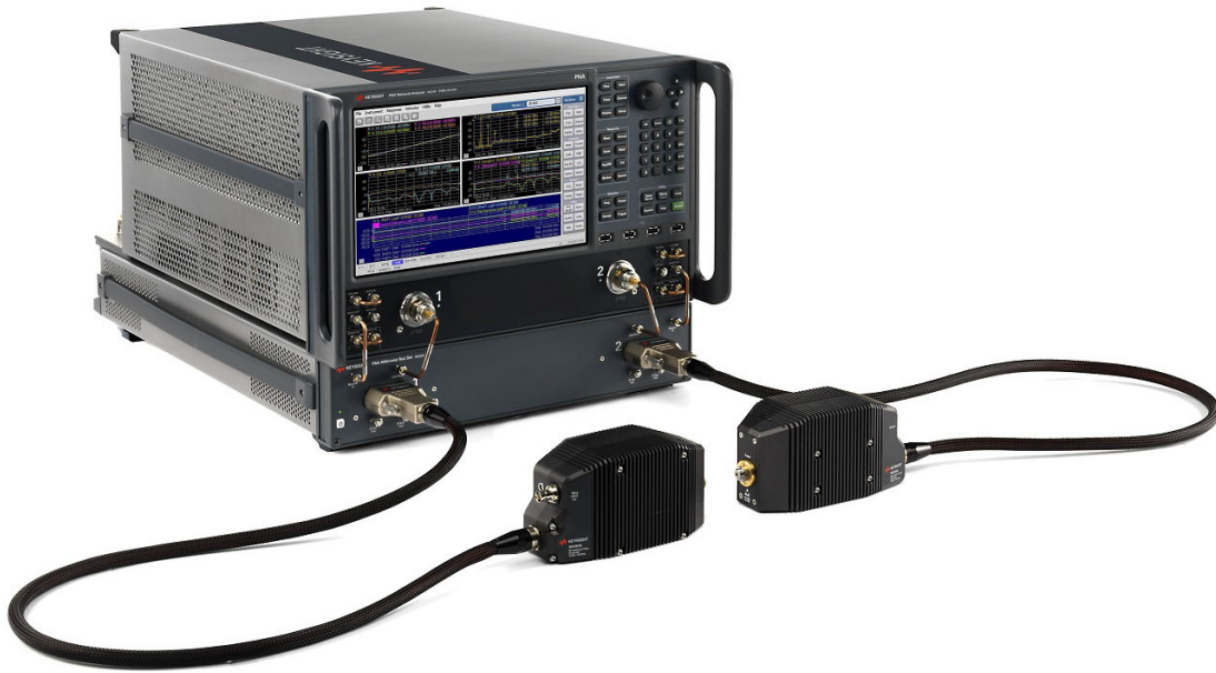
Figure 3-18 Cable Two Test Heads N5293/5AX03 to the N5292A. (Attach heads and torque cable screws to 8 in-lbs.)
